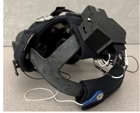
Fig. 8: Instrumented VR headset with 16 dry ExG electrodes (EEG, EMG, ECG, EOG) and a wireless bioamplifier.
