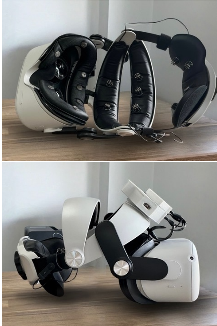
FIGURE 3.4 : Instrumented VR headset developed for this study.
